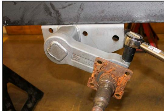
4. Using a thin, steel wedge, tap the wedge into the slot at the rear end of the torsion arm. This will expand the arm socket slightly and release the clamping pressure holding the old spindle in place.
