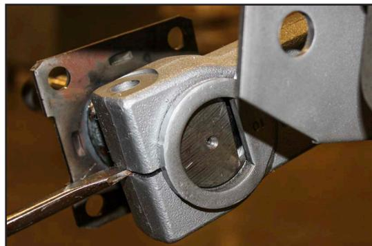
8. Push the spindle in until the shoulder butts up against the surface of the torsion arm.
