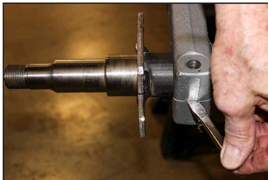
10. Use only the 1/2"-20 bolt included in the spindle replacement kit (bolt has adhesive thread locker already applied).
