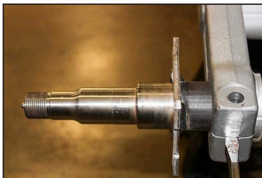
9. Remove the wedge and insert the 1/2"-20 clamp bolt (with lock washer installed) in from the top side of the torsion arm.
