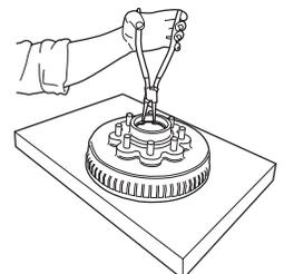
3. When replacing a Nev-R-Lube® bearing pack, the bore in the hub should be cleaned and inspected for visual damage (replace as necessary).
