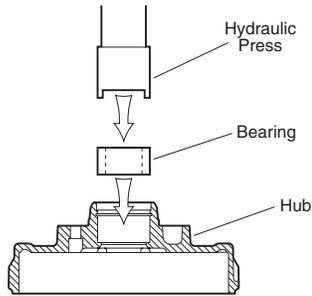
4. Install the new bearing using an arbor press fitted with a hollow or stepped punch face to press only on the outer housing of the bearing. Failure to follow procedure will damage the bearing and/or seals during installation. Press bearing until it seats against the backup shoulder machined into the hub.
