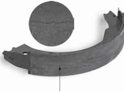
Acceptable Hairline Cracks
